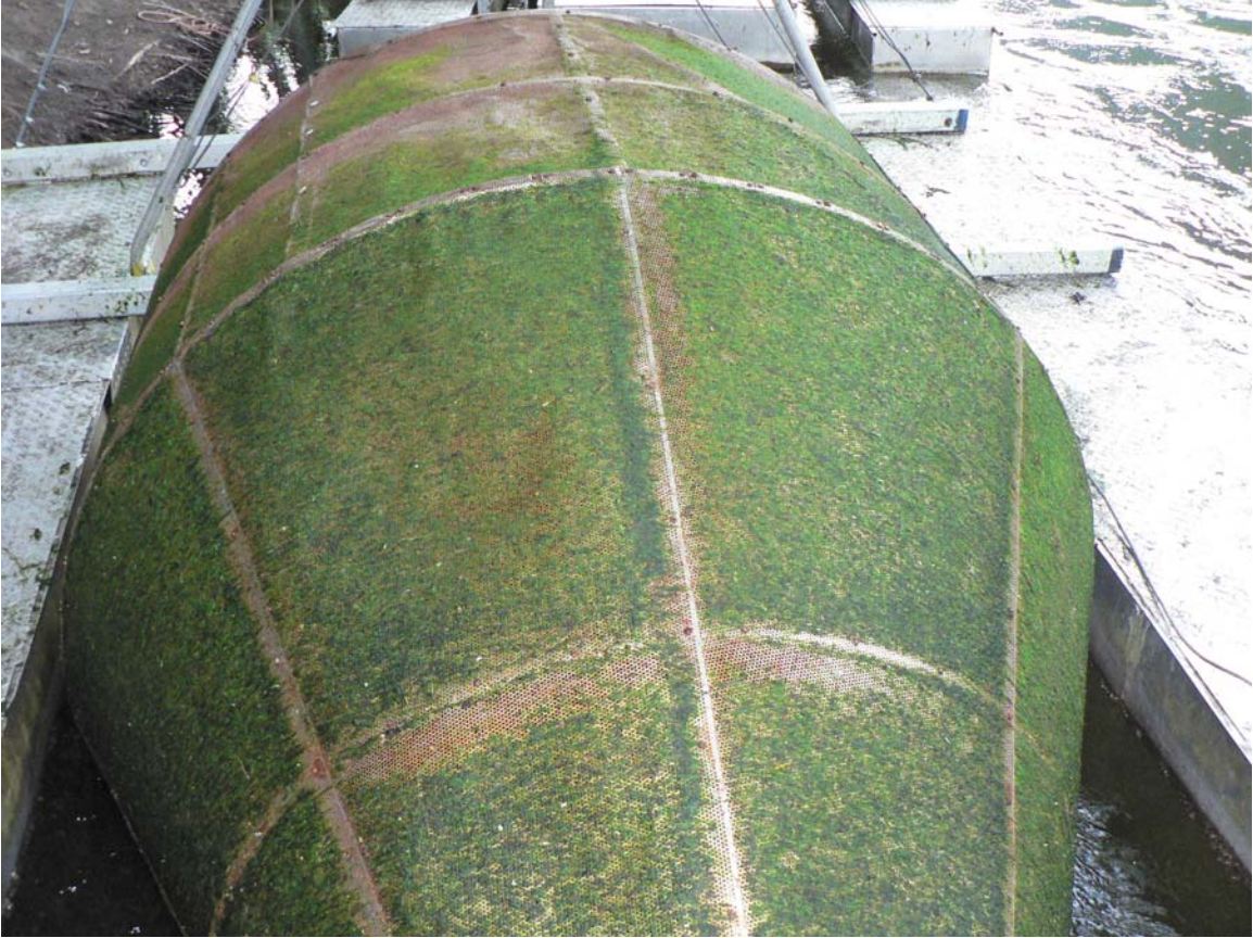
Figure 4. Photo showing 3 hours of algae build-up on drum of RST, May 17th, 2006.
